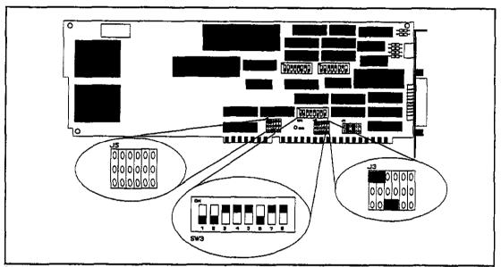
Figure 2-2 KPC-488.2TM Card Jumper and Switch Locations
