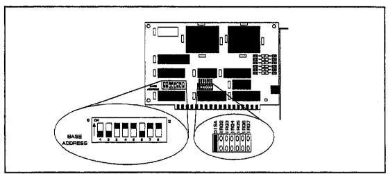
Figure 2-1 KPC-TM Card Jumper and Switch Locations.
