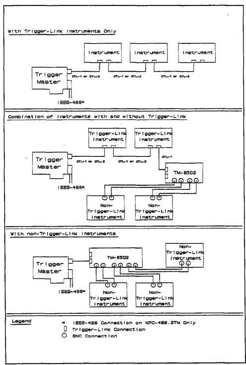
Figure 1-2 Trigger-Link Configuration Examples
