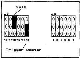
Figure 2-3 Jumper Blocks J5 and J3 Example
