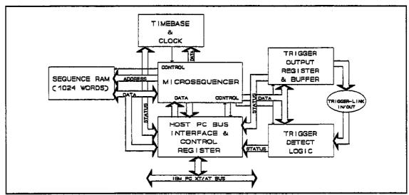
Figure 1-1 Trigger Master Block Diagram
